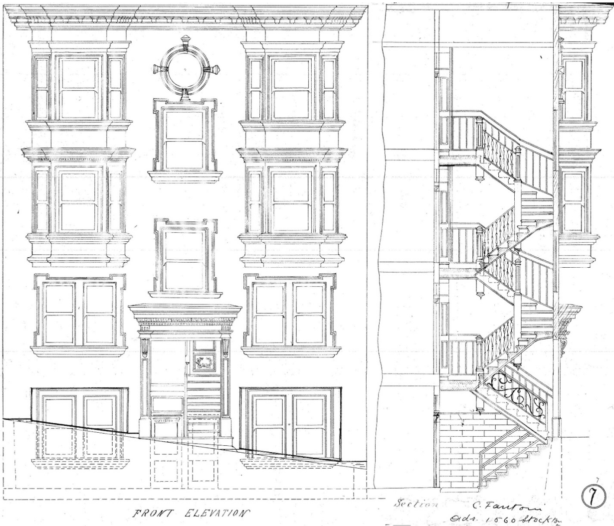
Figure 13 Original blueprints by Charles Fantoni, 1907, for a 3-floor Romeo Flats Building (6 flats) at 471-77 Vallejo St. (#660) showing front elevation and Romeo stair detail; Source: Northeast San Francisco Conservancy Archive (See Photo No. 40 of extant building)
